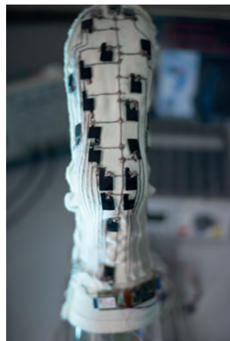
Fig. 3 Stocking with DES array to detect critical pressure load and prevent pressure sore
